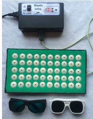
Figure 3. Device containing 50 LEDs ( 850 \pm 20 nm)
